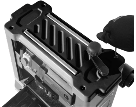
Fig. 13 – Removendo a tampa superior
